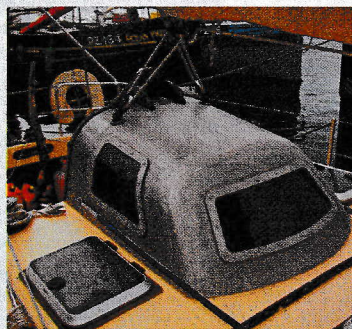
The companionway is covered by an aluminium doghouse. Note the two hatches either side to vent the steel hull in hot weather
