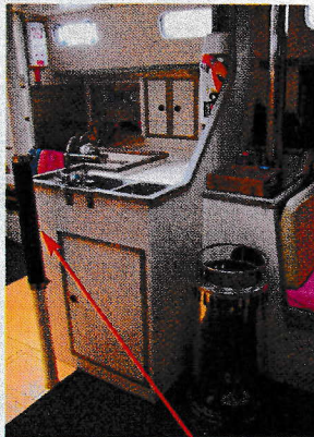
The rope for the retractable centreplate rises to the deck via a tube in the saloon. The tube has a removable rubber section for easy disassembly
