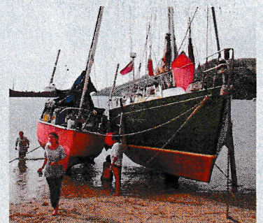
Lean on me. Norwegian Blue on a beach near the Panama Canal. You can see her multi-chine hull with the protruding keel box
